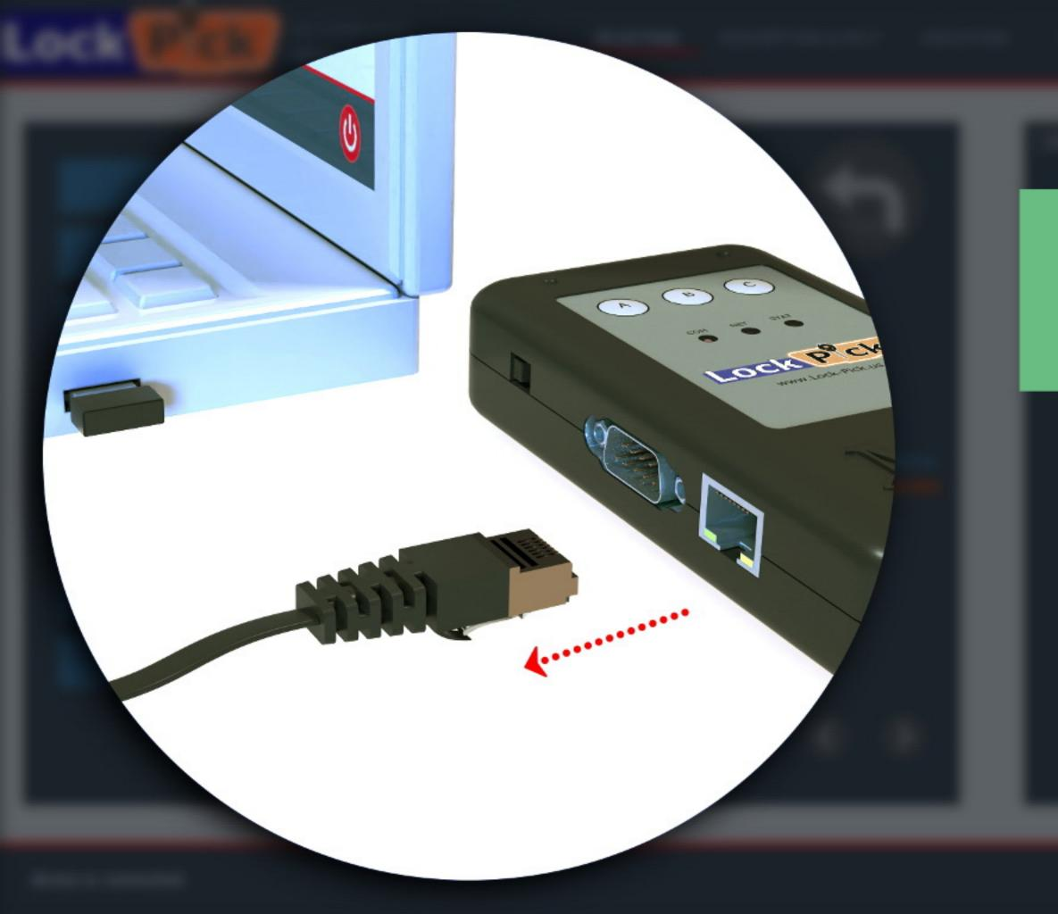
Removing the LAN cable will automatically switch the device from LAN to WIFI mode.
